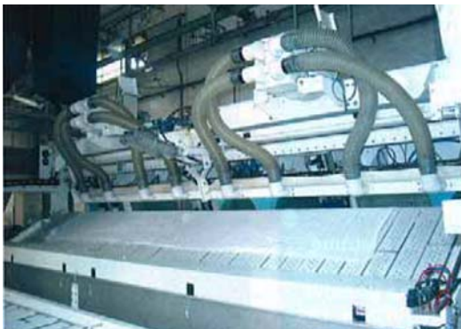
A suction system allows the sheet to be placed on the feeder table and to remove the cotton fluff by vacuum.
