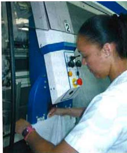
The operator inserts the street into the clamps without having to find the corners.
