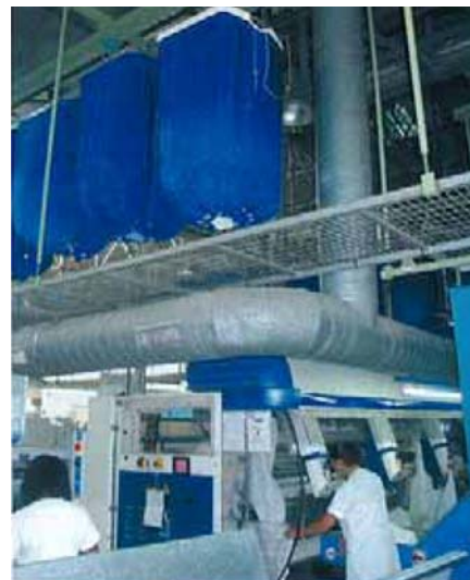
The shortage of space in terms of length and height has led to the choice of the Galaxy feeder.
